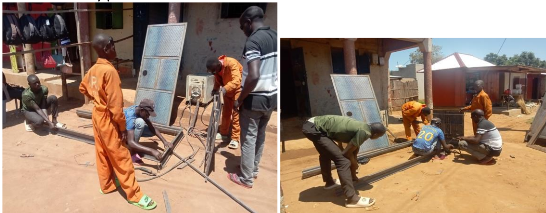
The youth at a welding workshop at Apado Welders learning how to set metallic door frame.
